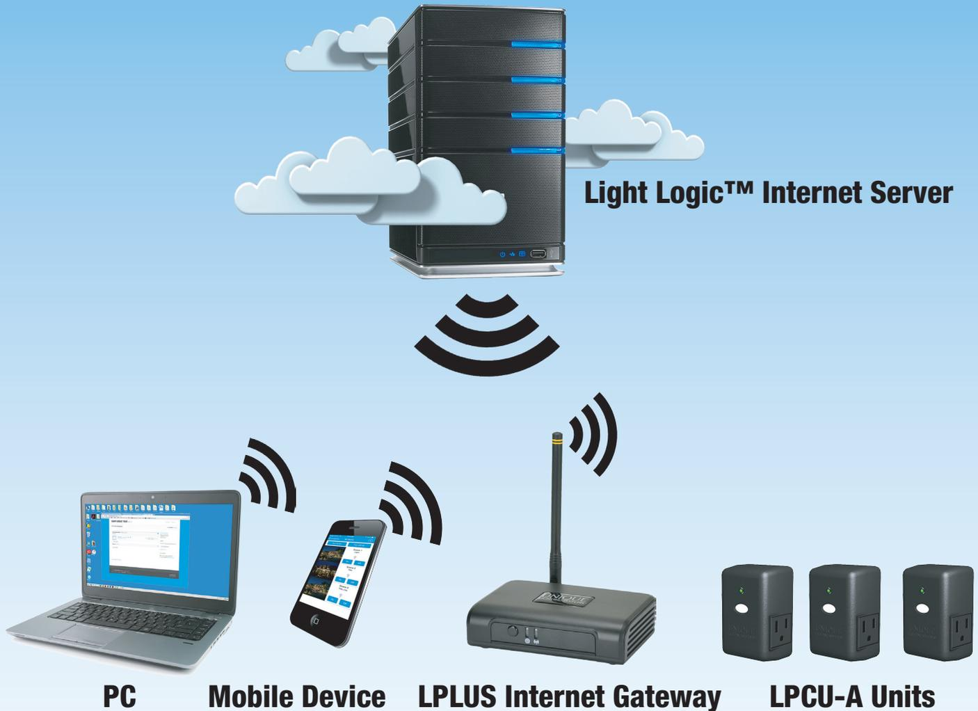
**PC** - Configure locations, scenes, schedules and other functional options using the PC at [www.lightlogicplus.com](http://www.lightlogicplus.com). The PC communicates with the LPLUS Internet Gateway via the Light Logic™ Internet Server.
