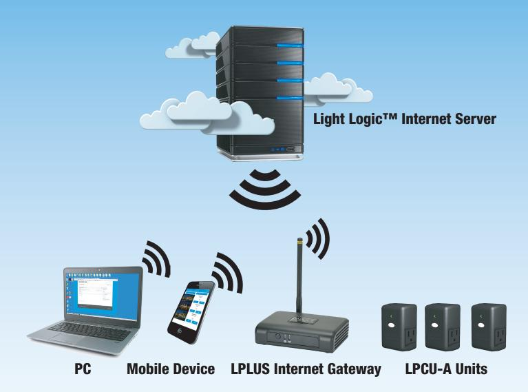
**PC** - Configure locations, scenes, schedules and other functional options using the PC at www.lightlogicplus.com. The PC communicates with the LPLUS Internet Gateway via the Light Logic<sup>™</sup> Internet Server.
