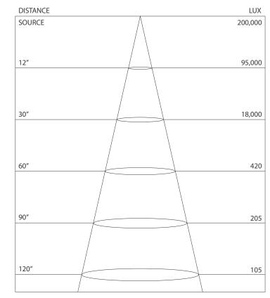
Note: The curves indicate the illuminated area and the average illumination when the luminaire is at different distances.
